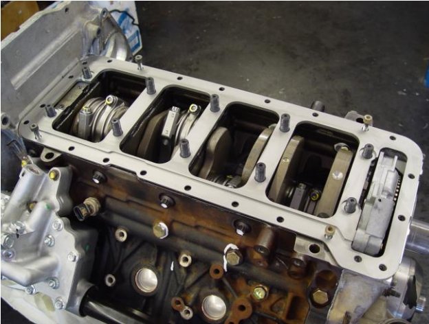
(3) APPLY A 1/16 INCH BEAD OF SILICONE (PERMATEX THE RIGHT STUFF) AND INSTALL GIRDL.
